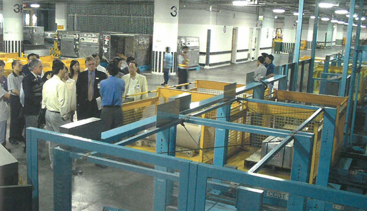
▲ The Bulk Cargo Distribution System is a sushi-bar style conveyor loop system that moves cargo between floors and workstations within SuperTerminal 1. 散貨分送系統是儼如壽司吧的散貨環迴輸送系統，貫通超級一號貨站各層和工作站。
