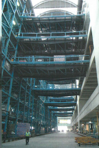
▶ The fully-automated Container Storage System has 3,500 storage positions. 全自動的航空貨箱貯存系統設有 3,500 個貯存位置。
